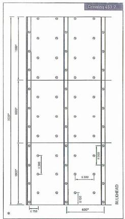
\* Dimensions may vary depending on structural design and size of insulation slab.
